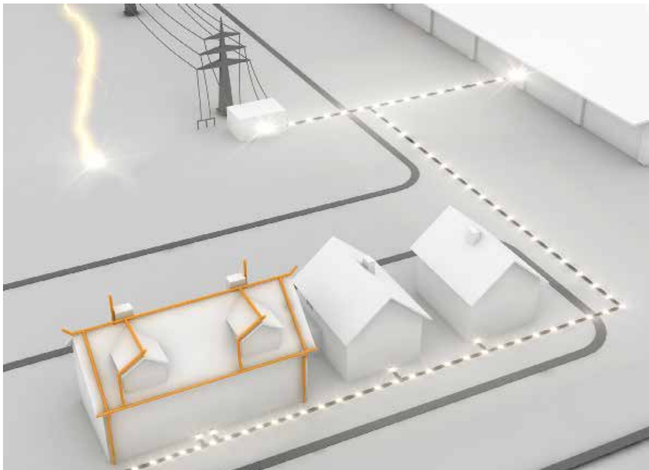
Fig. 1.14: Danger: galvanically coupled and line-carried surge voltage
