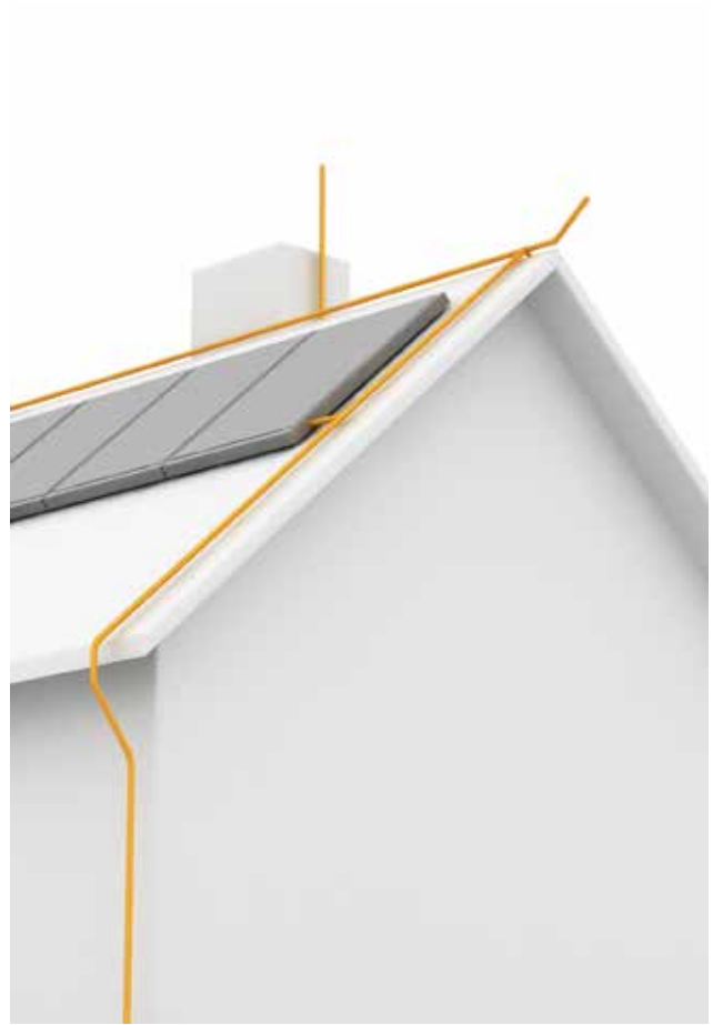
Figure 2.19: Direct connection of PV mounting frames to the lightning protection down-conductor system
