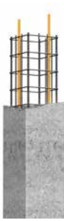
Figure 2.53: Example: use of reinforced concrete supports/down-conductor system
