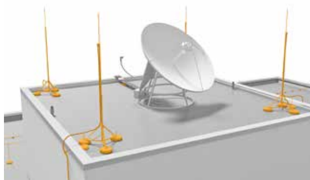
Figure 2.61: Isolated lightning protection with interception rods
